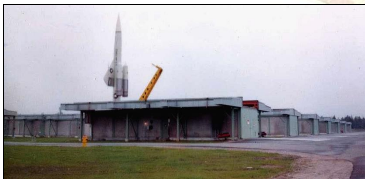
IM-99B BOMARC missile raised into firing position from its horizontal shelter at Raco (left & middle photos from http://www.airfields-freeman.com/MI/Airfields_MI_N.htm#raco )
